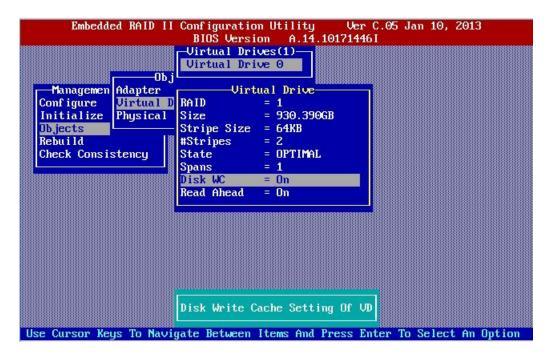
16. How do I enable/disable the logical drive write cache of Intel Onboard SATA ESRT2 RAID?
