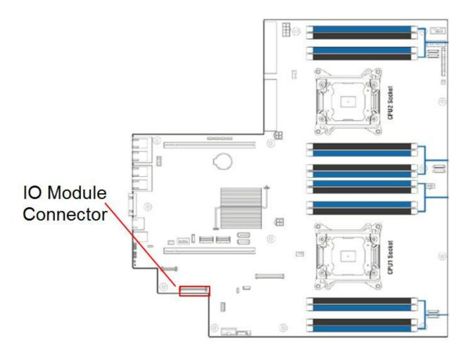
NOTE. IO Module connector is connected to CPU1.
