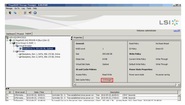
19. How do I enable/disable disk write cache of MegaRAID?
