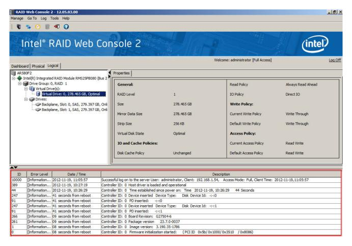
20. How do I save the event log of the integrated RAID Module RMS25CB040/RMS25CB080?
