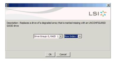
d. Right click the HDD marked as Offline and select Start Rebuild.
