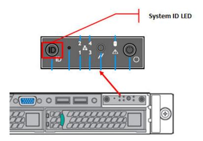
**ANSWER:** When servicing or performing maintenance tasks on Altos R360 F2, press the System ID button on the front panel to turn on System ID LED on the front and rear panels.
