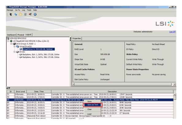
22. The MegaRAID is configured with 2 x HDD as RAID 1 without hot spare. But, when I removed one HDD and inserted the original HDD back, the RAID cannot be rebuilt automatically. In the RAID Utility, it indicates the HDD as (Foreign) Unconfigured Good.
