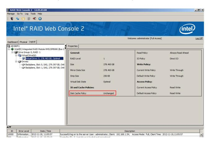
18. How do I enable/disable disk write cache of the integrated RAID Module RMS25CB040/RMS25CB080?
