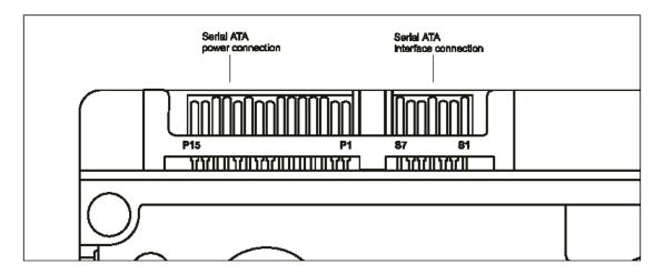
Below table identifies the pin definition of the SATA connectors and the corresponding signal names and signal functions (based on Western Digital SATA HDD).
