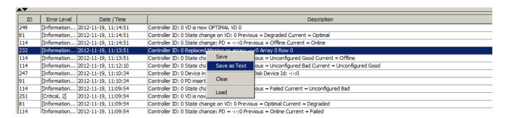
21. The integrated RAID Module RMS25CB040/RMS25CB080 is configured with 2 x HDD as RAID 1 without hot spare. But, when I removed one HDD and inserted the original HDD back, the RAID cannot be rebuilt automatically. In the RAID Utility, it indicates the HDD as (Foreign) Unconfigured Good.
