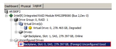
**ANSWER:** Please insert a new HDD which was not configured as RAID. Or, please install the original HDD into another RAID card and clear/delete its RAID configuration before you insert it into the degraded RAID.
